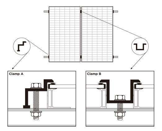
When choosing this type of clamp-mounting method, use at least four clamps on each module, two clamps should be attached on each long sides of the module (for portrait orientation) or each short sides of the module (for landscape orientation). Depending on local wind and snow loads, additional clamps may be required to ensure that modules can bear the load.
