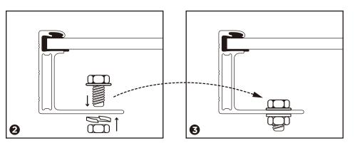
Secure the module in each mounting location with an M8 bolt and a flat washer, spring washer and nut as shown in Figure 1 and tighten to a torque of 16-20 N.m(140-180lbf.in.).
